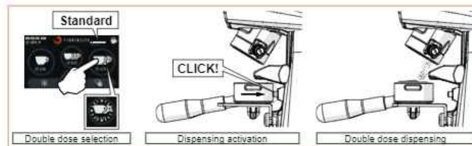
Fig. 12 - Double dose dispensing in 'Standard' mode.
